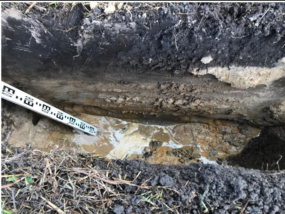
TP10 encountered 0.25m of topsoil overlying sand. Groundwater was encountered at 0.8m.
